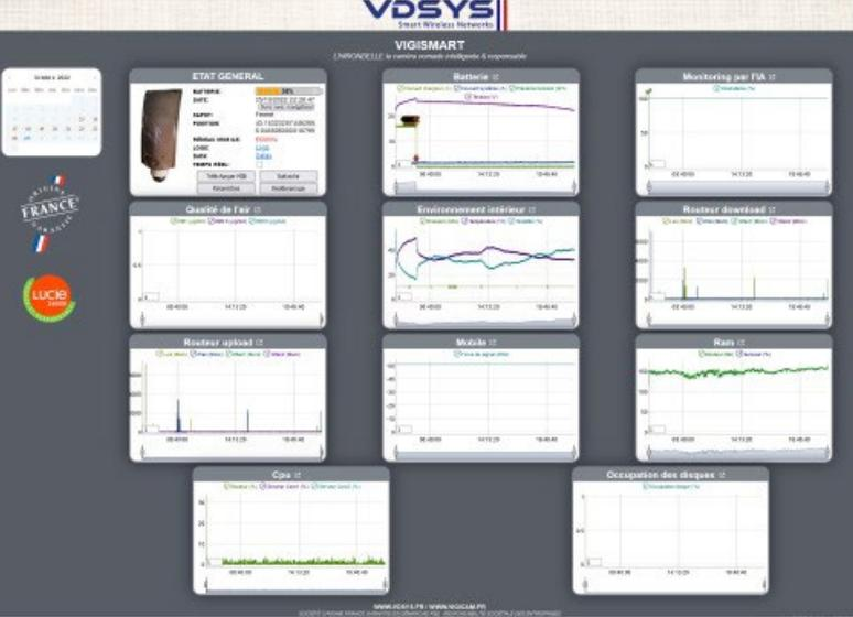
The screenshot displays the VIGISMART monitoring interface. It features a central 'ETAT GENERAL' (General Status) panel with a router image and key statistics. Surrounding this are several line graphs and bar charts, including 'Router #1', 'Monitoring par FA', 'Router download', 'Router upload', 'Moyenne', 'Rais', and 'Coe'. The interface is branded with 'VDSYS Smart Wireless Networks' and includes logos for 'FRANCE' and 'LUCIE'.
